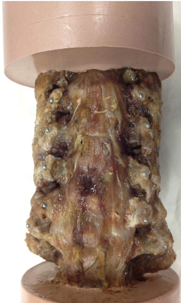
Figure 21: Specimen ready to be tested with C2 and T1 levels potted in Bondo.
